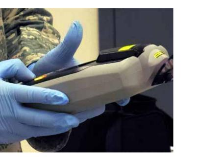
Field-portable technology allows border control agents to conduct confirmatory tests on an unknown substance in a matter of seconds. This hand-held spectrometer can test for narcotics, explosives, drugs and other chemicals.
